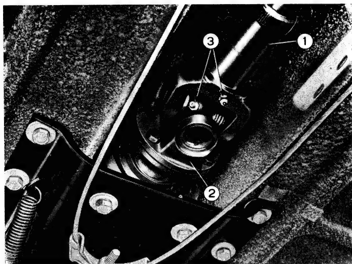
Fig. 130. - Detail of prop shaft center universal joint.
