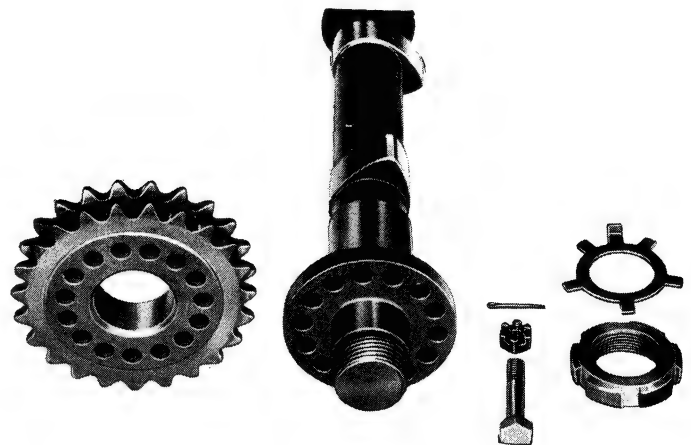
Fig. 65. - Flanged camshaft with sprocket, location screw, nut, cotter pin, adjuster ring and lockplate (engine 118 B.000).
